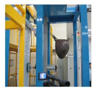
• The walls of the lift must withstand 1000N without any permanent deformation of a minimum of 1mm and without elastic deformation of a minimum of 15mm.
